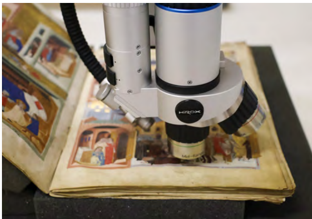
Analysis of the colour layer with a digital microscope.
