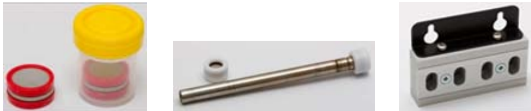
Examples of passive air samplers and a dosimeter. Photo: Marie Benešová
